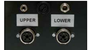
Rear-panel showing photo-detectors connectors.
